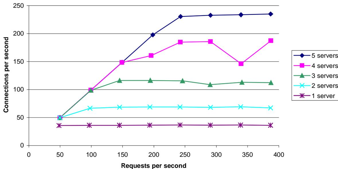
Figure 8. Rate.d performance for different cluster sizes
