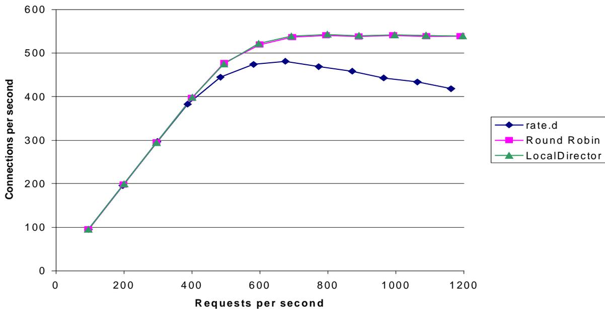
Figure 11. Throughput comparison for workload without CGI requests
