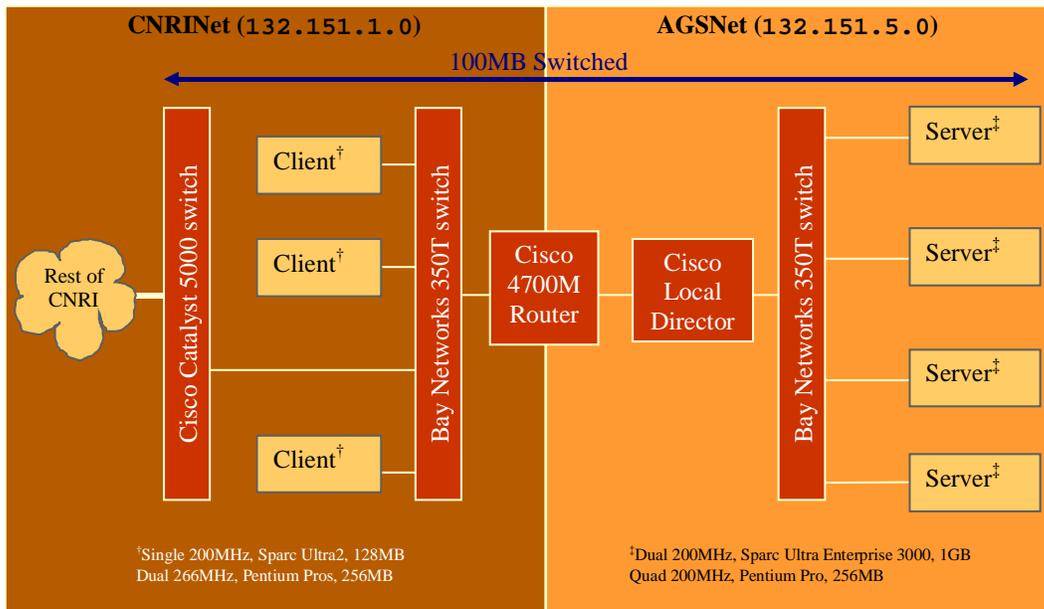
Figure 4. Network architecture of the AGS test environment
